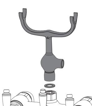
Fit the hose to the cradle & handset using the small sealing washers.
